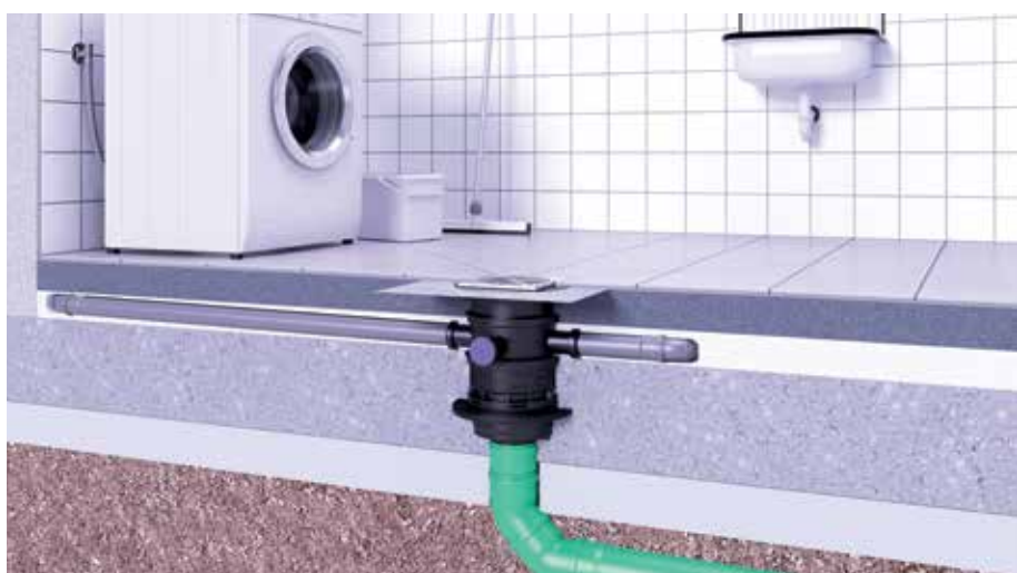
Installation with waterproofing against groundwater
