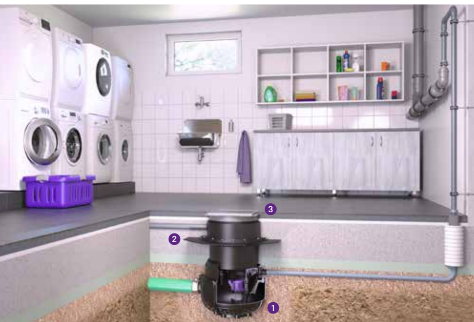
1 Lifting station 2 Extension section with flange 3 Cover with integrated inlet
