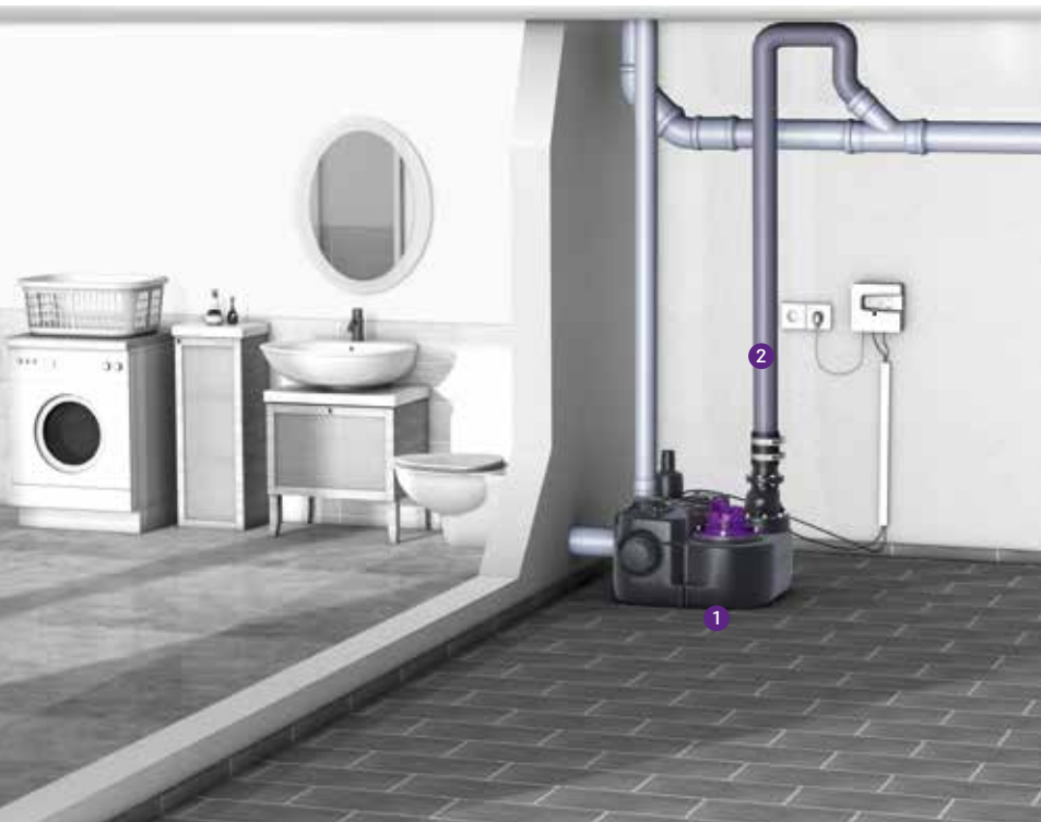
1 Lifting station 2 Pressure pipe
